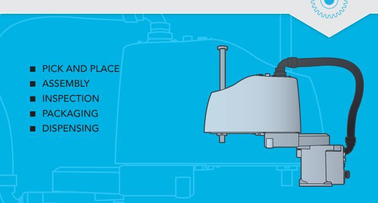
Selective Compliance Assembly (or Articulated) Robot Arm. Slightly compliant in X-Y, horizontal, plane, but rigid in Z (vertical) direction. Generally a 4-axis unit, with most under 13lb (6kg) payload capacity and 25" (650mm) of reach.
